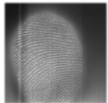
500ppi FBI Spec Fingerprint Reader on Flexible Polyimide
